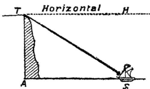
(i.) In calculating the horizontal distance  $AS$  of a ship  $S$  from the point  $A$ , vertically beneath the point of observation  $T$ , *the angle of depression  $HTS$*  is observed through which it is necessary to depress the instrument in order to sight on  $S$ . Then, since  $TH$  and  $AS$  are parallel,  $\angle AST = \angle STH$  (by Prop. 2 (ii.)), and this, with the measurement of  $AT$ , enables the triangle to be drawn, or calculated. (See Prop. 5.)
