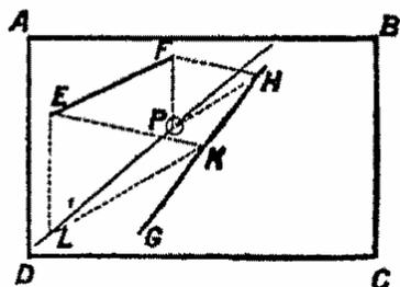
Let  $ABCD$  be a drawing-board, and let  $EF$  and  $GH$  be two lines upon it which intersect beyond the limits of the board.
