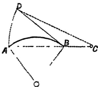
Graphical determination of the length of a circular arc.
