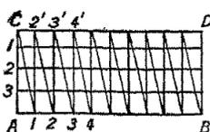
The diagonal scale enables us to subdivide a small distance very accurately. Thus, if  $AB$  be a line, which it is required to divide into 40 equal parts, say. Divide  $AB$  into 10 equal parts, and set up a perpendicular  $AC$  of any
