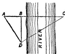
To measure the width of a river, &c., indirectly.
