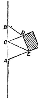
2. Let it be required to determine an angle  $ABC$  with a chain only. Produce  $CB$  to any convenient length  $BD$ . Set off the same or any other convenient length  $BE$  along  $BA$ , and measure  $DE$ . Then the  $\triangle DBE$  is determined,
