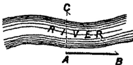
Suppose it required to measure the width between  $A$  and  $C$  on opposite banks of a river. Measure a baseline  $AB$  on one side of the river, and at its extremities measure the angles  $ABC$ ,  $CAB$ . Then the width  $AC$  is determined either by drawing to scale or by calculation (Prop. 5).
