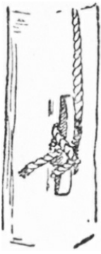
THIS IS A CLEAT WITH A HALYARD BELAYED ON IT
